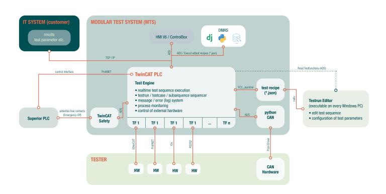
At the core of the architecture is the test engine, which runs the test hardware. The test recipe editor is used for test run configuration. The head system handles the data management between the customer's system and the tester.
