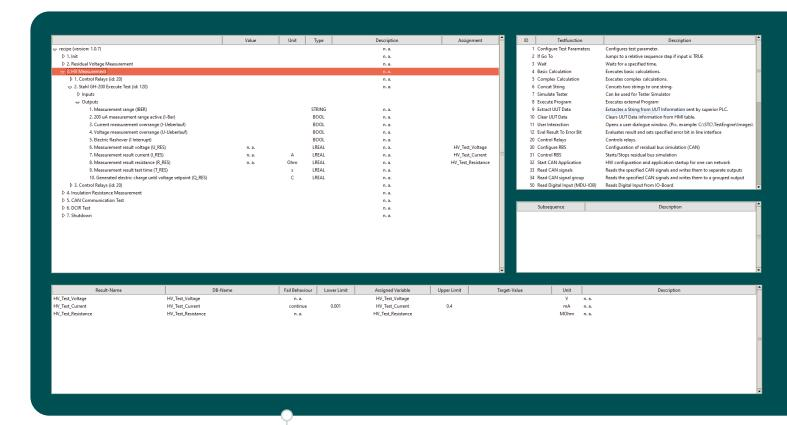
The test sequences can be defined in the top left window. All available test functions are listed in the top right part of the screen. Shown below that are so-called subsequences, within which recurring test sequences can be defined and then inserted into the overall test sequence in the form of a macro. The bottom part of the screen shows the configuration of the result entries. These can be made available to the customer's IT system for archiving once the test is complete.
